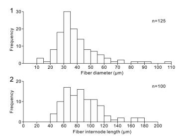
**Figure 4.** Vermiform fiber dimensions measured from Figure 3.6. (1) Histogram of vermiform fiber widths. (2) Histogram of vermiform fiber network internode distance.
